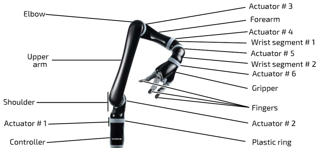
Figure 1: Robot components
